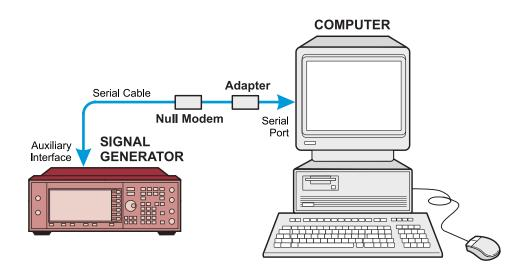
Set the RS-232 parameters in the signal generator. Press Utility > HP-IB/RS-232 and set as follows:
